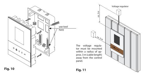
Place the control panel directly in front of the housing base and pay attention to the correct orientation. Plug in the connection cable with the RJ10 plug to the control panel. Now press the control panel carefully into the housing base until the fastening tabs lock securely. Make sure the control panel sits reliably in the base part.
