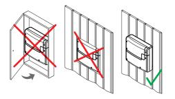
Attention: The relay box may not be installed in a closed switch cabinet or behind a wooden panelling!
