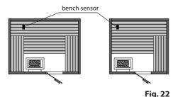
The bench sensor is connected with a 3-core wire silicone cable with RJ10 plug to one of the free sensor bus jacks in the relay box, as shown on the fig. 23. Cable connection to the board inside sensor are shown on fig. 24.
