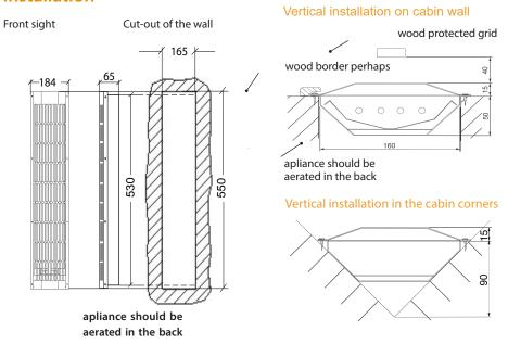
Attention! Make sure to provide sufficient air circulation around the radiator. The space above the radiator must not be blocked, so that the warm air may rise freely. Risk of fire!
